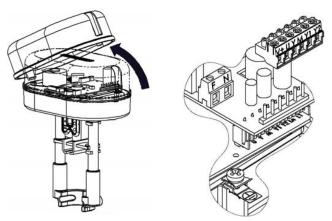
Note: To avoid damage to electronic components caused by the PCB bending, do not press too much while fi xing the terminal block.
