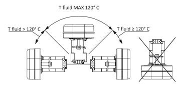
To mount the actuator on to a valve, position the valve stem to the bottom of its travel, slide the actuator onto the valve neck, adjusting with the manual override the screw jack position so the square nut on the valve spindle fi ts into the groove on the cross bar. Then slide the brace into the groove on the valve neck and secure the nuts.
