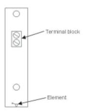
When options are selected, connections are made using terminals on the PCB as shown.
