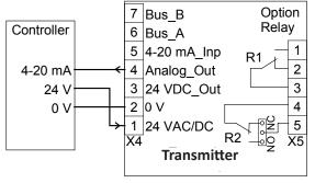
Two-wire connection 4 - 20 mA output signal without options Do not connect power supply at this pin! 0VDC, 24 VAC, or 0 VAC will destroy the detector!
