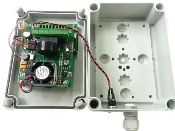
Cable gland for RS232 or RS485 connection
