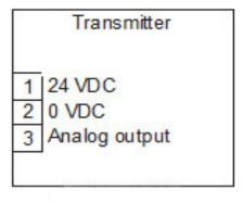
Terminal 2 i only for 2-10Vdc signal = 3-wire 4-20mA two-wire loop powered
